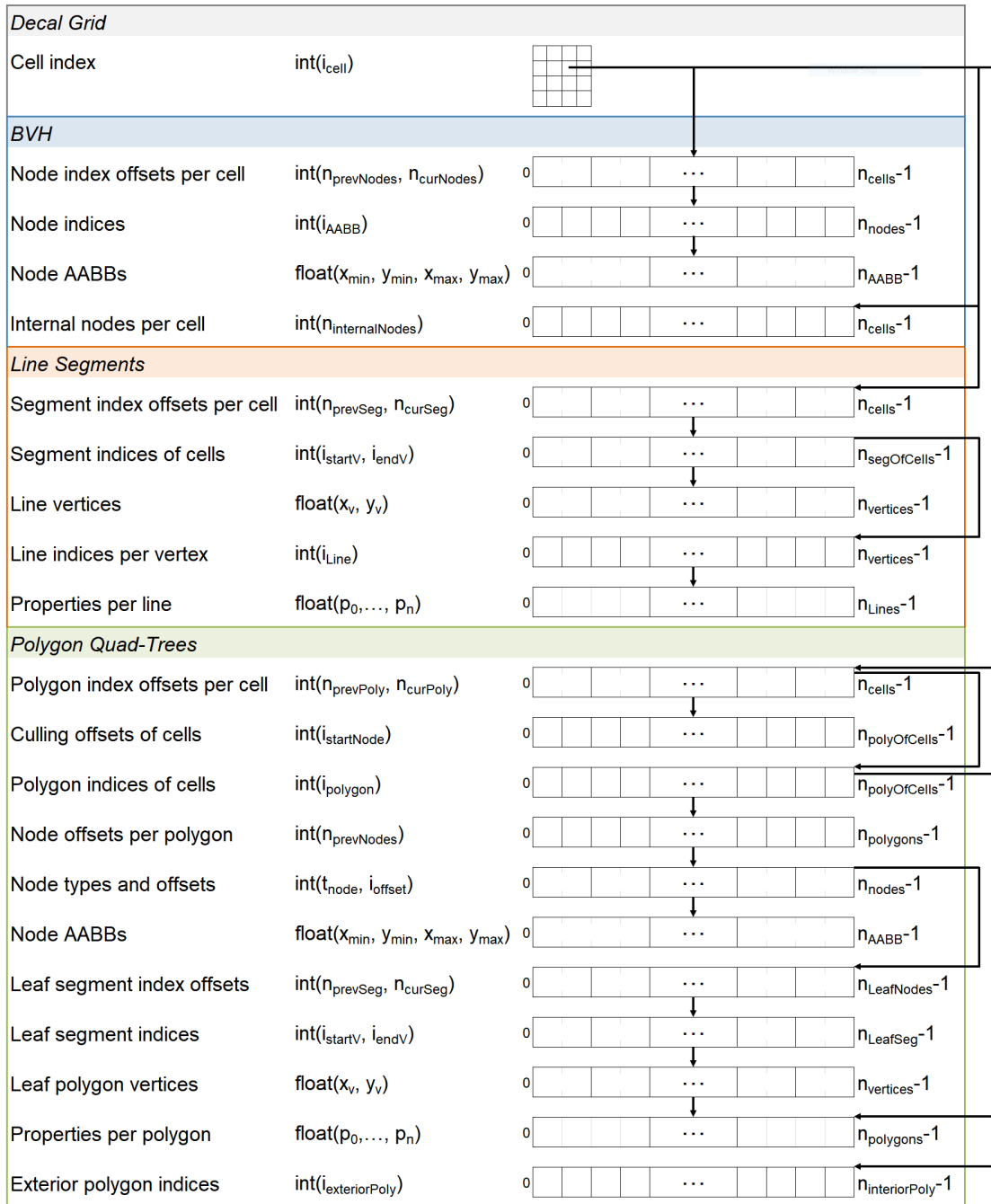
Figure 4.2: The data that are necessary for rendering of static lines and polygons with data types and sizes. They contain indices i , numbers of objects n , and positions with xy -coordinates and are stored in shader storage buffers. Decal grid and BVH data are required for both decal types, for lines also segment data and for interior and exterior polygons also quad-tree data are necessary.
