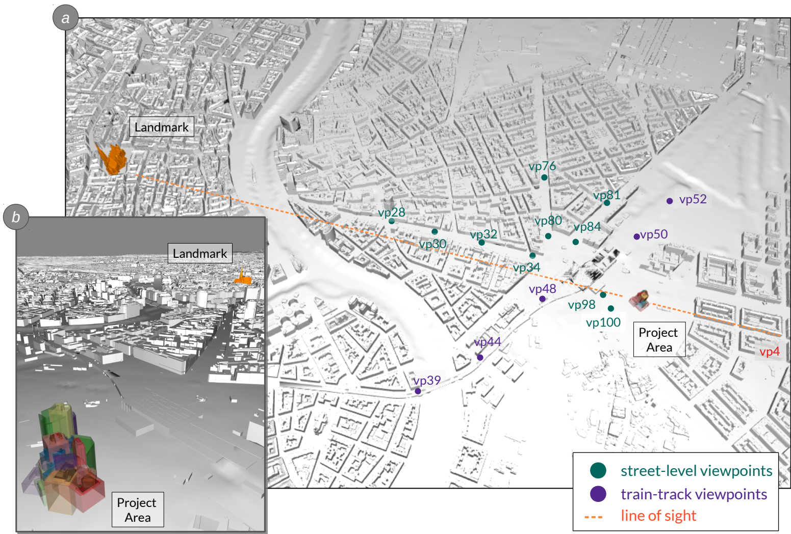
Figure 3.4: (a) Bird's-eye and (b) close up view, both showing the project area near the railway station with all building candidates and a landmark (orange). Further, we show exemplary viewpoints at street level and on the train tracks, as well as a line of sight.
