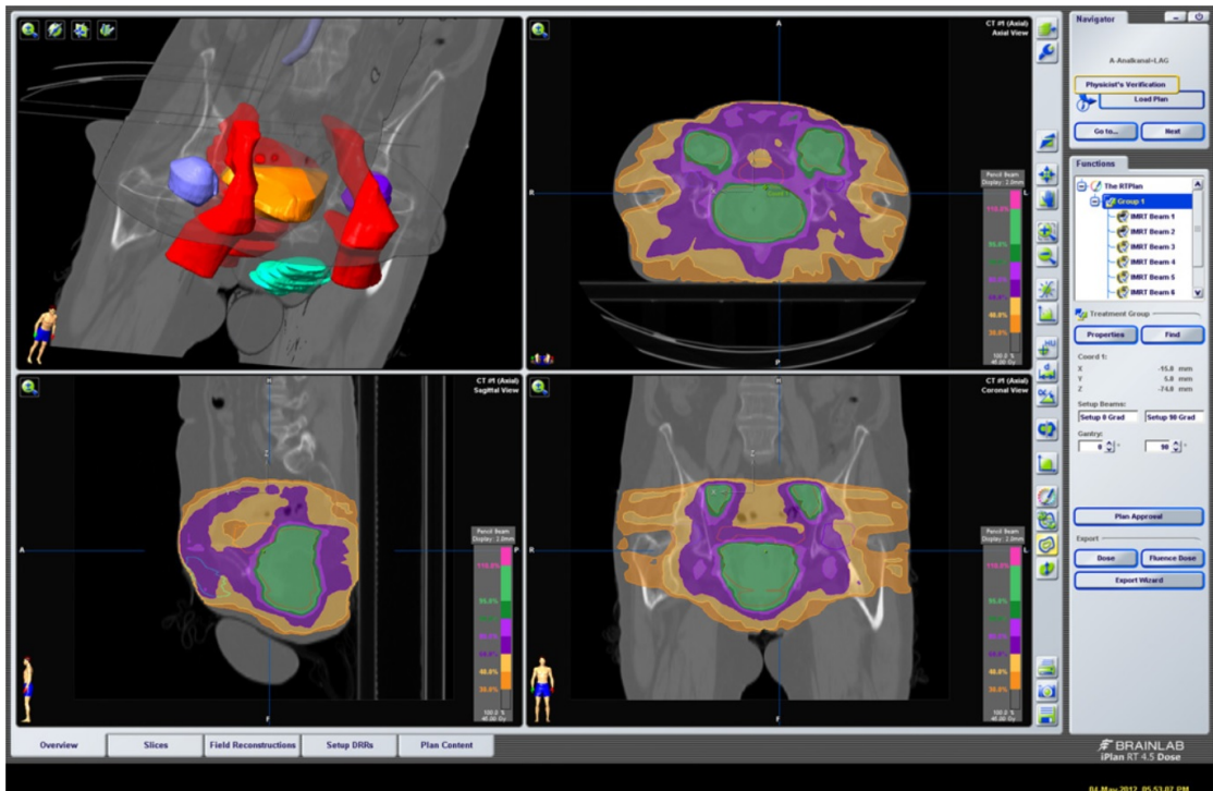
Figure 2.3: The axial, sagittal and coronal slices together with a 3D overview to evaluate the simulated dose distribution used to treat prostate cancer. The 3D overview (upper left) shows the previously segmented anatomical structures along with the three orthogonal slices. The slice views employ isolines and colored regions to display the dose distribution as percentage of the target radiation in the tumor (Courtesy of Mathias Walke, Department of Radiation Treatment Planning, University of Magdeburg, taken from the book of Preim and Botha [PB13]).
